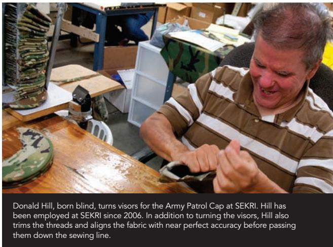
Donald Hill, born blind, turns visors for the Army Patrol Cap at SEKRI. Hill has been employed at SEKRI since 2006. In addition to turning the visors, Hill also trims the threads and aligns the fabric with near perfect accuracy before passing them down the sewing line.
